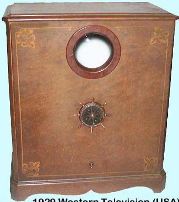
1929 Western Television (USA) Scanning Disc Television
